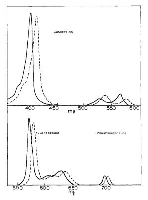
Figure 1. Absorption spectra (top) of zinc etioporphyrin in cyclohexane (----) and pyridine (---) at 28° and emission spectra (bottom) of zinc etioporphyrin in EPA (----) and in EPA with pyridine (- - -) at 77°K.
