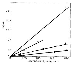
Figure 2. Typical Stern-Volmer plots for quenching of zinc and magnesium etioporphyrin fluorescence by nitrobenzene:  $\phi_0/\phi$ , the relative fluorescence intensity in the absence and presence of nitrobenzene; •, zinc etioporphyrin in piperidine; •, zinc etioporphyrin in ethanol; O, magnesium etioporphyrin in piperidine; , magnesium etioporphyrin in methylcyclohexane.
